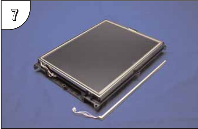
The above shows the backlight bulb completely removed from its guide in the panel's main electronics housing. (Only one bulb shown.)
