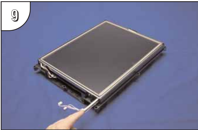
Position the replacement bulb so that the opening in its three-sided gold colored reflector faces toward the LCD touch screen. Using gentle pressure, slide the bulb into the guide until it is flush with end of guide.
