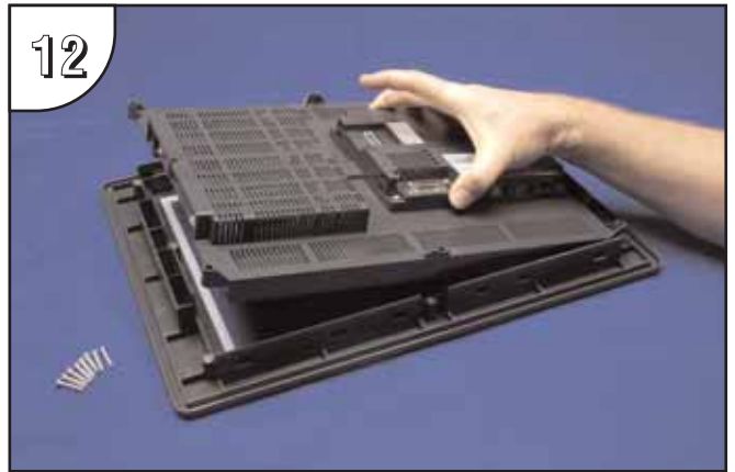
Position the touch panel's main electronics housing into the front bezel so that the flat ribbon cable on the housing matches up with the recess in the front bezel. Insert the eight screws and tighten to a maximum of 70 oz-in [0.5 Nm].
