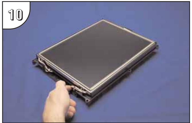
Plug each backlight bulb's two power cable connectors back into their respective circuit board connectors. Each bulb's two connectors are keyed to prevent mismatching.
