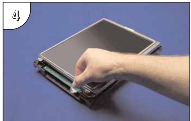
4 Carefully lift the bulb's wires out of the wire guides so they are free from obstructions.
