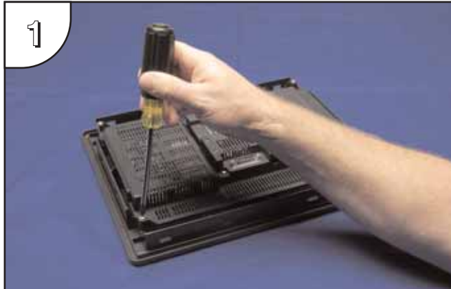
1 With power disconnected, use a #2 Phillips screwdriver to remove the four outer screws holding the touch panel's main electronics housing to the front bezel.
