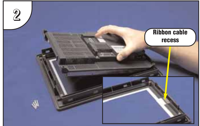
2 Lift the touch panel's main electronics housing from the front bezel. Set the front bezel and four screws to the side. Observe the ribbon cable recess on the front bezel (see detail) for use in re-assembling the panel.
