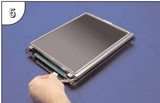
5 Unplug the backlight bulb's power cable connector from the circuit board connector.
