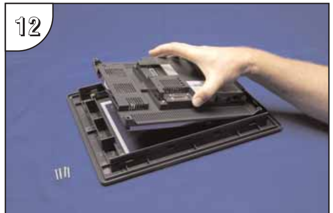
12 Position the touch panel's main electronics housing into the front bezel so that the flat ribbon cable on the housing matches up with the recess in the front bezel. Insert the four screws and tighten to a maximum of 70 oz-in [0.5 Nm].
