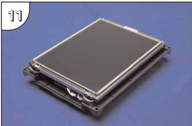
11 Gently position each backlight bulb's wires back into their respective wire guides to help clear any obstructions when inserting the panel's main electronics housing back into the front bezel. Position any excess wire length in between the printed circuit board and the LCD to prevent it from becoming pinched between the housing and bezel.
