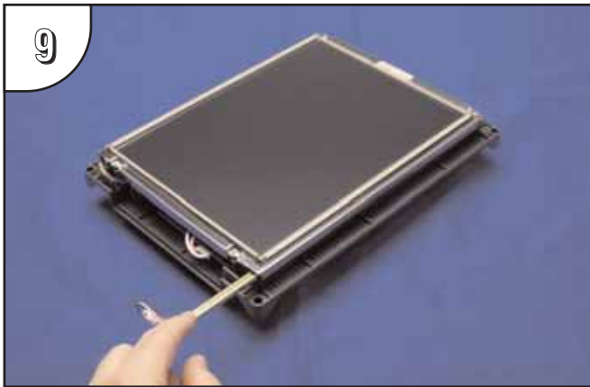
9 Position the replacement bulb so that the opening in its three-sided gold colored reflector faces toward the LCD touch screen. Using gentle pressure, slide the bulb into the guide until the retaining clip locks.
